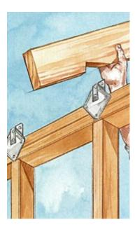
Fasten the bottom ends of the common rafters to the wall plates with metal anchors.
